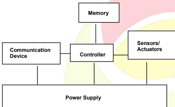
A WSN consists of various sensor nodes to measure the data from the environment which is communicated to other nodes and to the base station [23]. The base station stores the sensor data and transmits the data to a remote system through Internet or some other communication medium such as Zigbee. The architecture of a WSN is shown in Fig 2.
