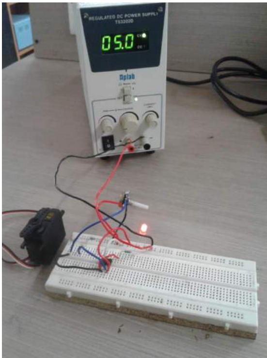
Fig 7: LED glows due to obstacle
