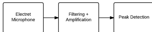
Noise Sensor Functional Level Diagram.
