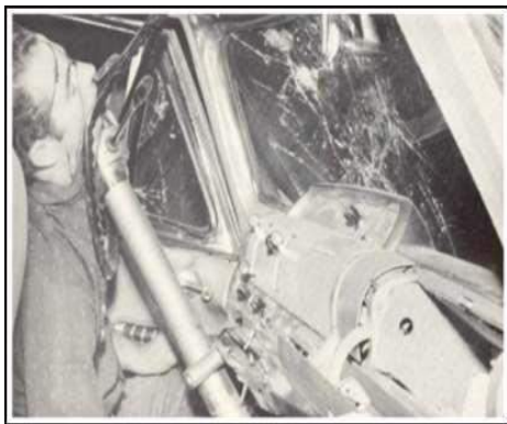
FIGURE-2.1-Steering column collapse
