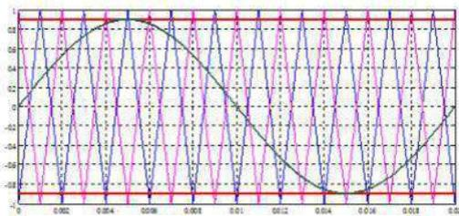
Fig.4: Simple Boost control of ZSI
