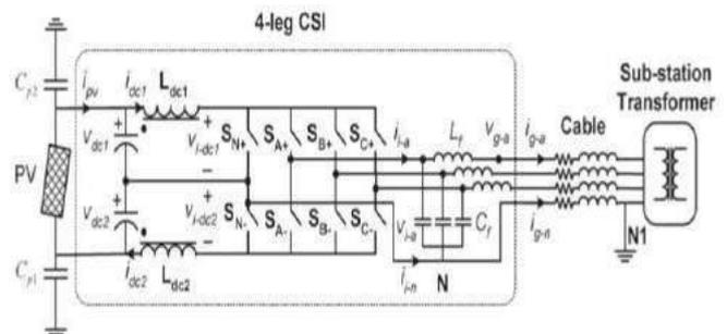
Fig. 6. Circuit diagram of Conventional 4-leg CSI
