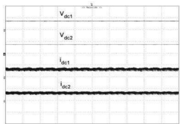
Fig. 7. Experimental results: dc capacitor voltages  $v_{dc1}$  and  $v_{dc2}$  (200 V/div) and dc inductor currents  $i_{dc1}$  and  $i_{dc2}$  (10 A/div). X-axis: time (10 ms/div).
