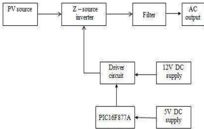
Fig.10: Block diagram of Proposed ZSI
