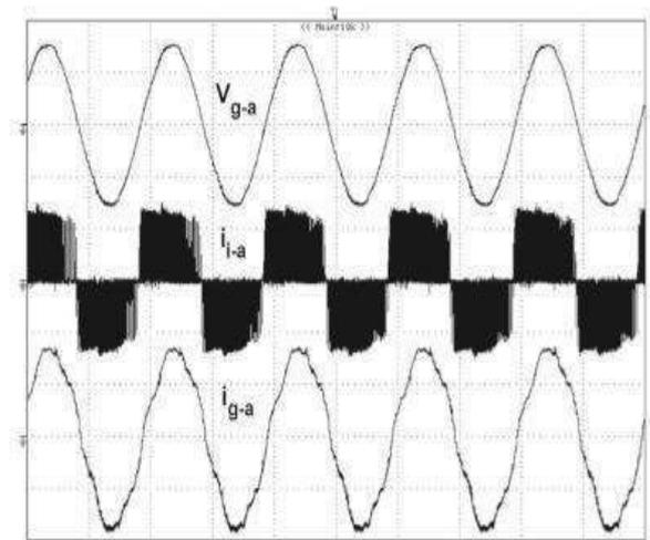
Fig. 8. Experimental results: ac phase-a voltage  $v_{g-a}$  (200 V/div), inverter PWM current  $i_{i-a}$  (5 A/div), and grid current  $i_{g-a}$  (2 A/div). X-axis: time (10 ms/div).
