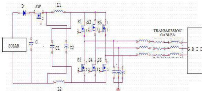
Fig.11: Circuit diagram of Proposed ZSI
