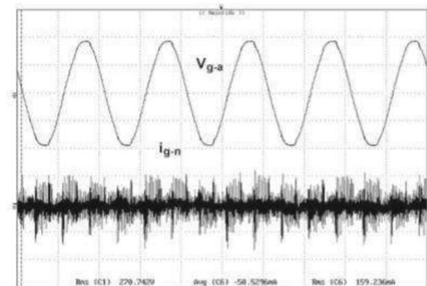
Fig. 9. Experimental results of the conventional scheme: phase-a voltage  $v_{g-a}$  (200 V/div) and neutral current  $i_{g-n}$  (0.5 A/div). X-axis: time (10 ms/div).
