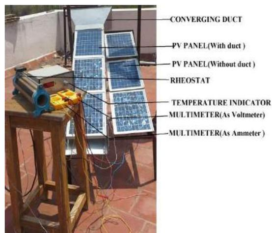
Figure.6 Photographic view of experimental setup
