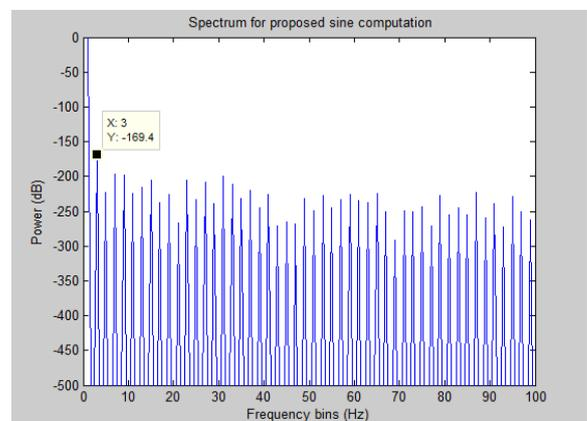
Fig. 9. Spectrum of the proposed DDFS using piecewise linearization with four uniform segments
