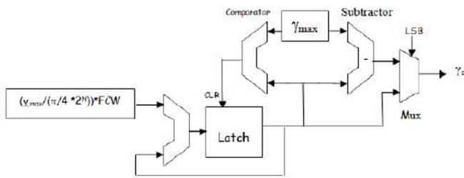
Fig. 5. Block Diagram of sine  $\gamma$  Accumulator
