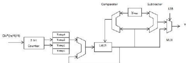
Fig. 6. Block Diagram of cosine  $\gamma$  Accumulator
