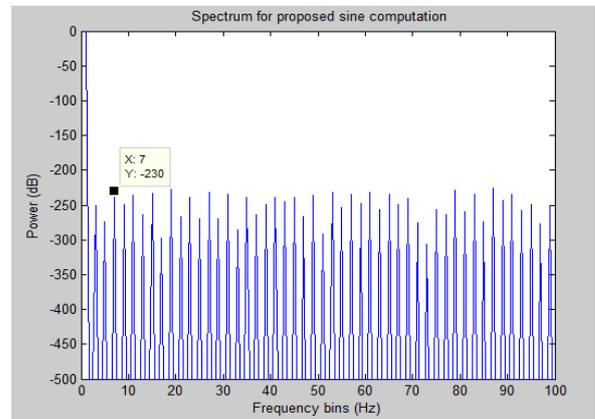
Fig. 7. Spectrum of the proposed DDFS using LUT for  $\gamma$  values
