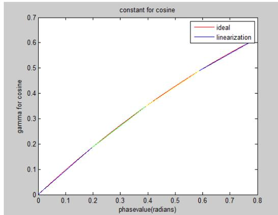
Fig. 3. Piecewise linearization of theoretical  $\gamma_c$  values with four uniform segments
