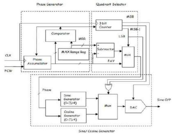
Fig. 4. Block Diagram of Proposed DDFS
