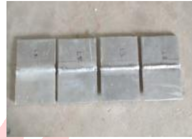
Fig.3. Specimen after MIG welding
