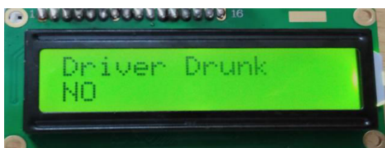
Fig -10: LCD Display on “Not Driver Drunk”
