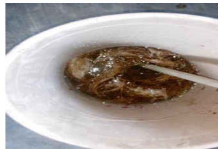
Fig2.3 Surface Treatment With NaOH
