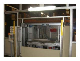
The roads will take in to the Mother tank for dosing for chrome process and transfer pumps for chrome and etch process Anodes for hard chromium bath Cathode 1 Cathode for etching bath. The roads have handling by using Transport equipment. In addition to the proximity switches, mechanical actuated safety switches are used for each transporter which provides anti-collision protection limitation for vertical movement. When these switches are actuated the corresponding drive is interrupted.
