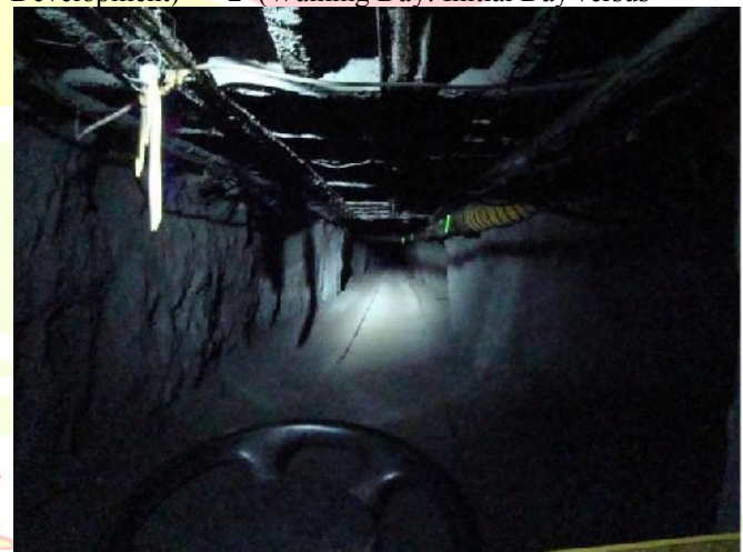
Fig.1. Circular beam spot of the Standard cap lamp used at the field test site. The photograph was taken at the NIOSH Safety Research Coal Mine.
