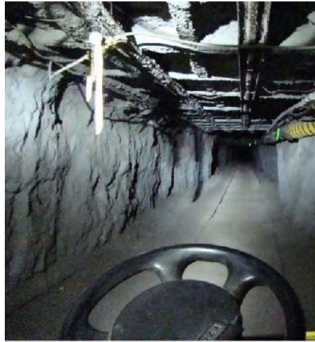
Fig.2. Light distribution of the NIOSH LED cap lamp. The photograph was Taken at the NIOSH Safety Research Coal Mine.
