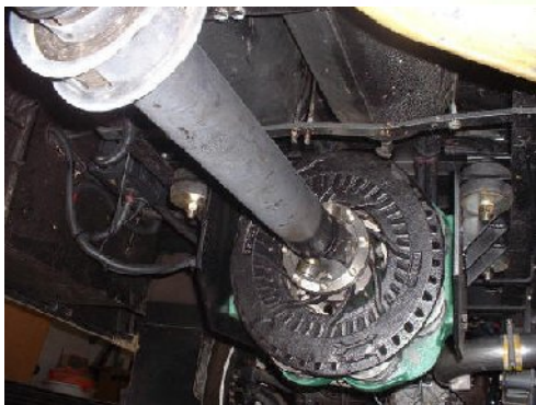
Fig. 3. Retarder installed on drive
