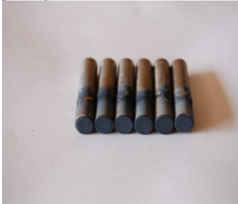
Fig. 4. AISI 304 stainless steel Pin materials
