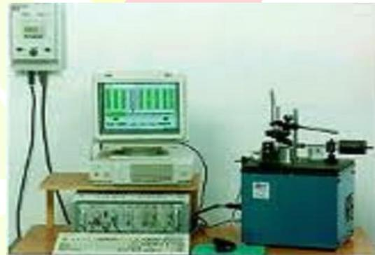
Fig. 3. Pin-on-disc apparatus for wear testing.
