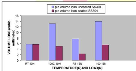
Fig. 9 Pin volume loss with respect to temp for coated and uncoated AISI 304 stainless steel.
