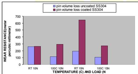
Fig. 10 Wear resistance with respect to temp for coated and uncoated AISI 304 stainless steel.
