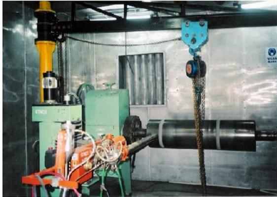
Fig.2. D-Gun method for thermal spray coating.
