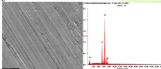
Fig. 11 SEM image and EDAX of uncoated AISI 304 stainless steel.
