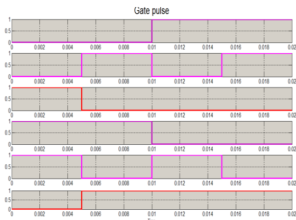
Fig.5. Pulse pattern of fundamental frequency switching
