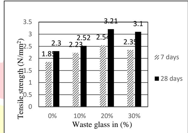
Fig.3 - Variation of Tensile Strength of Cylinders
