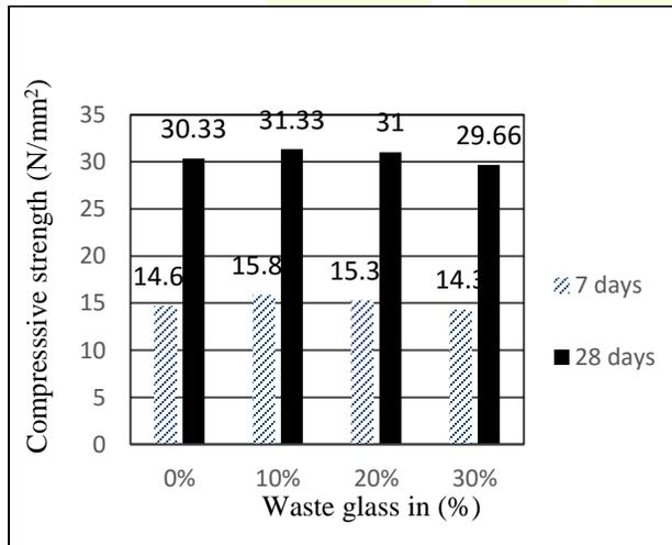
Fig.2- Variation of Compressive Strength of cubes
