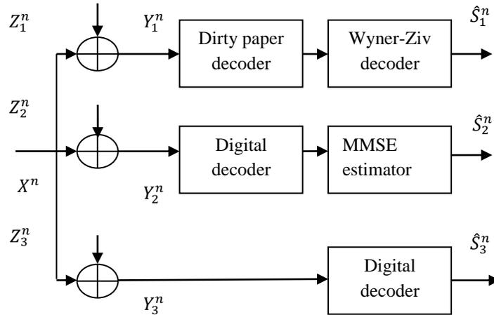
Fig.5. Decoder for broadcasting three Gaussian components over an average power limited Gaussian broadcast channel.
