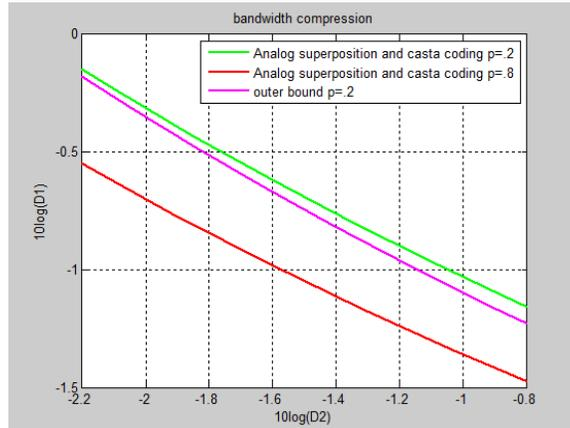
Fig.6. Distortion region for broadcasting bivariate Gaussian source with bandwidth compression.
