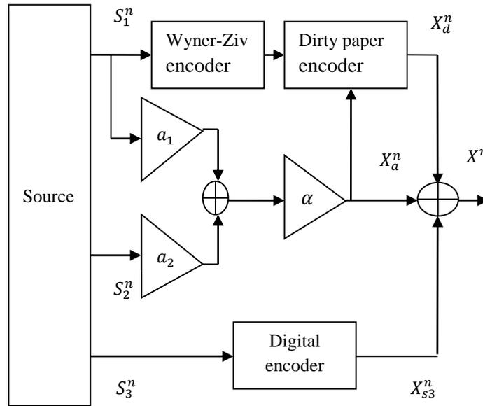
Fig.4. Encoder for transmitting three Gaussian sources over an average power limited Gaussian broadcast channel.
