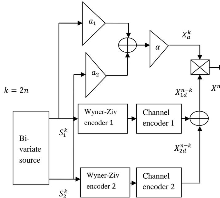
Fig.3. Encoder for bandwidth Expansion.
