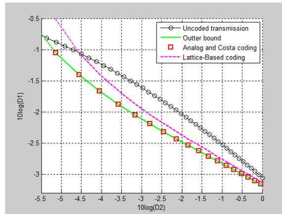
Fig.9. Comparing distortion region of broadcasting bivariate Gaussian source over power limited Gaussian broadcast channel using different coding scheme.
