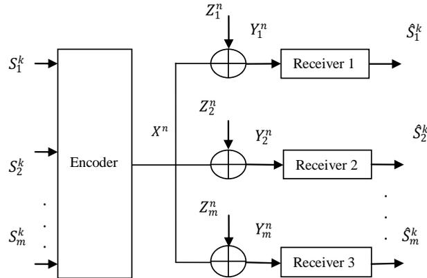
Fig.1. Broadcasting correlated Gaussian sources over a power limited Gaussian broadcast channel. Receiver  $i$  aims to reconstruct its source component with distortion  $D_i$ .
