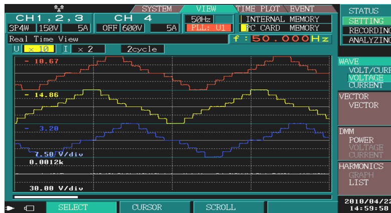
Fig 9. Line to Line voltage waveform of 5-level DCMLI in Power Quality Analyzer
