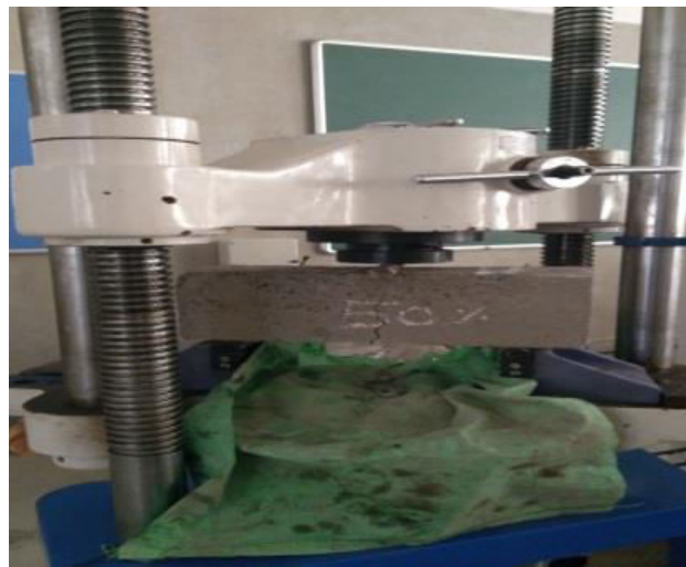
Fig.5 Indirect Tensile Strength setup
