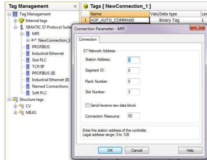
Fig.6 Connection between WinCC and AS (Automation System) using MPI
