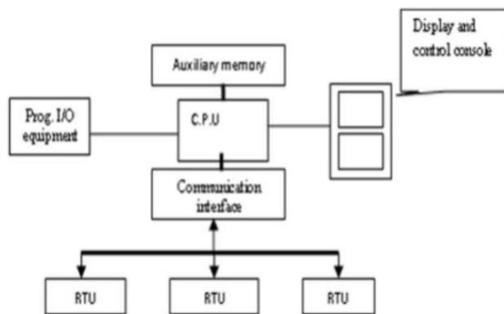
Fig.5 SCADA System with Single Computer
