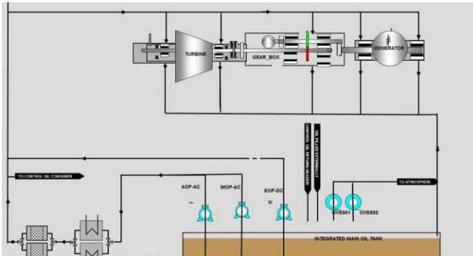
Fig.9 HMI developed for Lube Oil system in WinCC Flexible
