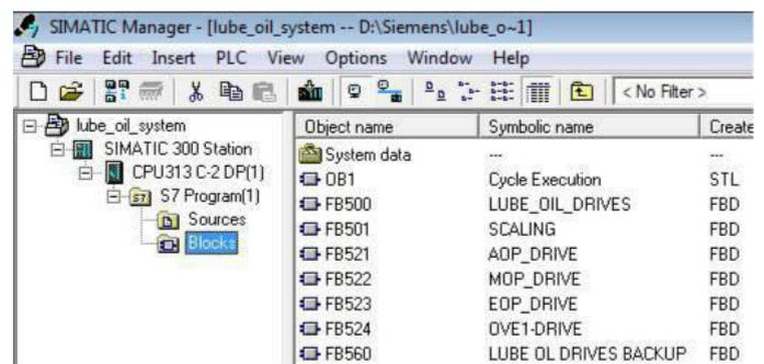
Fig.2 SIMATIC Manger Project Structure
