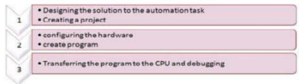
Fig.1 Basic Procedure for STEP7
