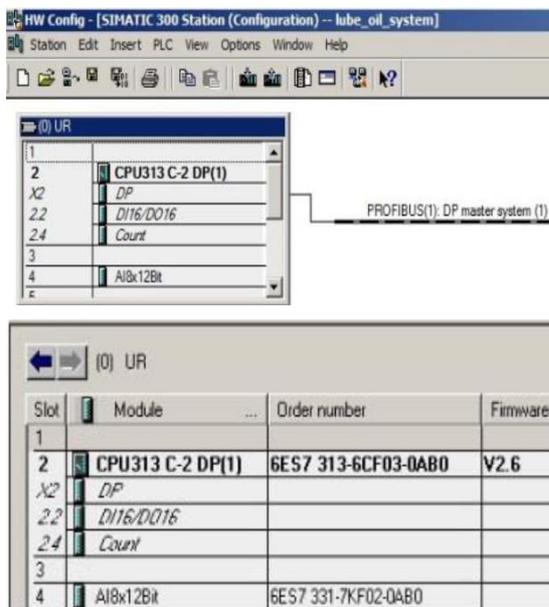
Fig.3 Hardware Configuration
