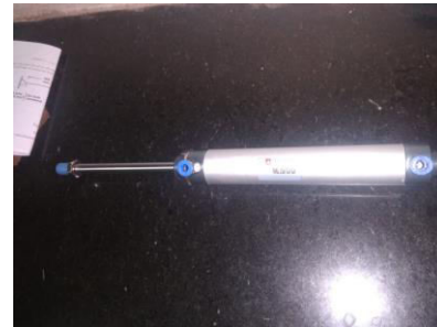
Fig 4.2 Pneumatic cylinder (25*100mm) & (32*200mm)
