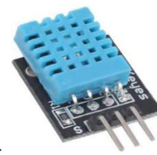
Fig 2: Temperature and Humidity sensor
