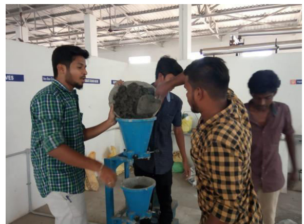
Fig no.2 Compaction factor test
