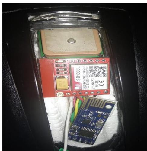
Wire wrap board is used for housing components to make a circuit for compactness, simplicity of servicing and ease of interconnection which is later embedded inside the helmet.
