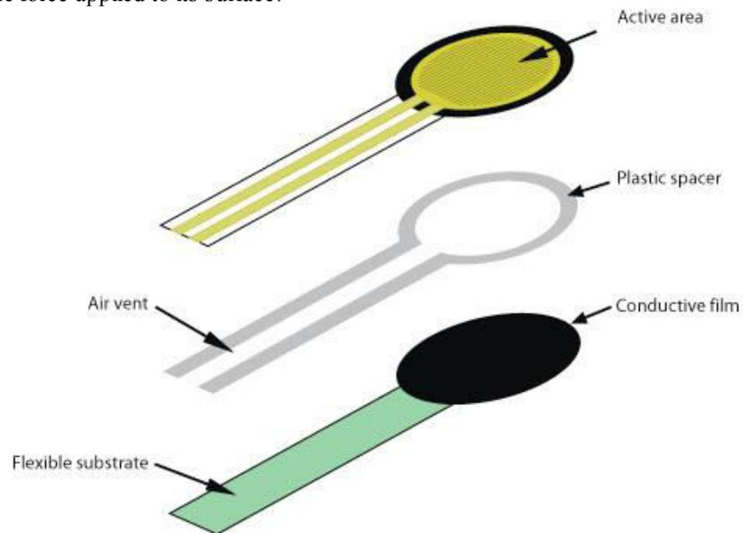
If force is applied to a surface of sensing film, then the particles touches the conducting electrodes and thus resistance of the film changes. There are several resistive based sensors but force sensing resistors operate satisfactorily in difficult environments and also require a simple interface compared to other resistive based sensors.
