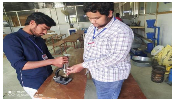
Fig 3: testing for normal consistency & Setting times of cement.
