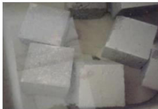
Fig 8. Curing Concrete Cubes
