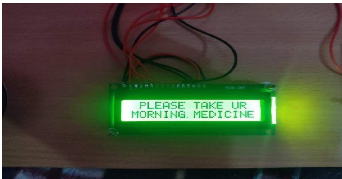
Fig 4.LCD display for taking morning medicine
