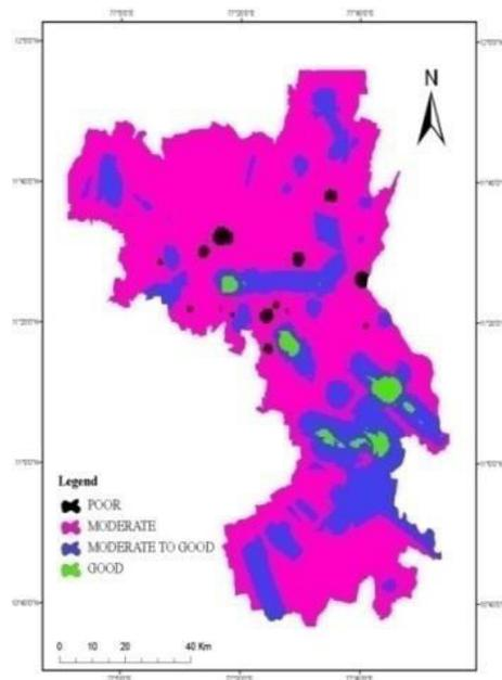
**Figure 4. Weighted Overlay of Lineament Density and Depth to Basement Maps**
