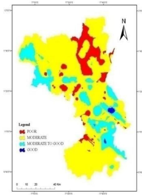
**Figure 5. Weighted Overlay of Lineament Density, Depth to Basement and Weathered Layer Maps**
