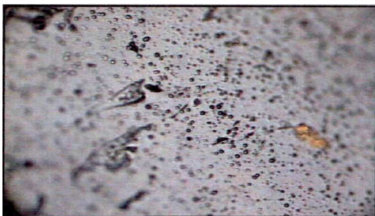
Figure 1. Micrograph of MoS 2 Single crystals used as a photo electrode
