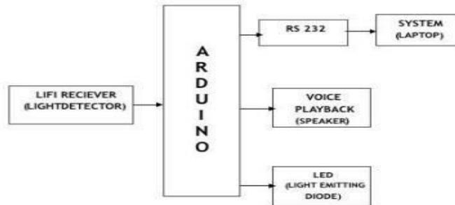
Figure 3. Receiver Block diagram
