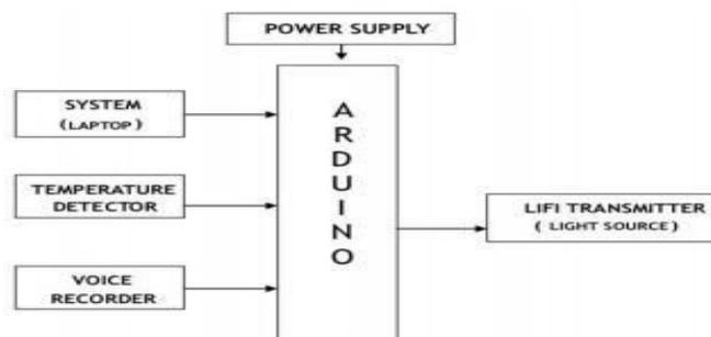
Figure 2. Transmitter Block diagram
