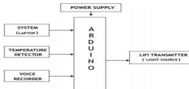
Figure 2. Transmitter Block diagram
